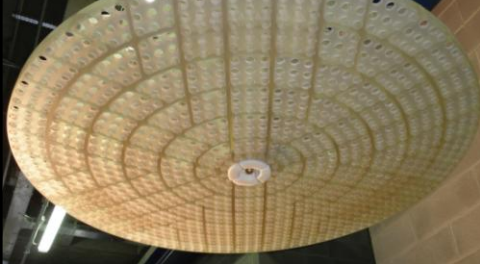
1.1m Zerodur shell, in manufacturing
