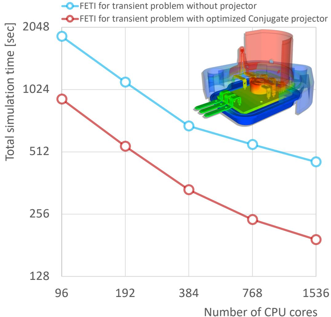
Still is possible to decrease the computational time by hardware optimization of the nonlinear steps, matrix assembler vectorization
